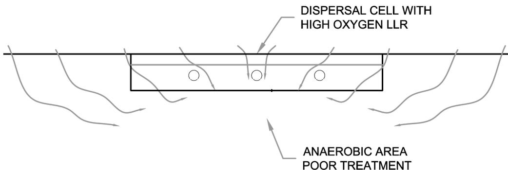
The maximum permitted effluent load per meter length of cell can be calculated. However, a simpler method was needed to address this and in BC we use two maximum LLR ranges to represent the “oxygen LLR” for a system.
