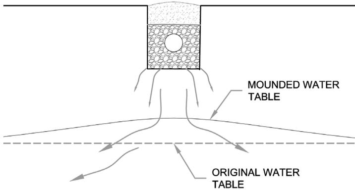
On a sloping site, the head pressure comes from a combination of the slope and the mound, and so the mound will be smaller as the slope gets steeper.
