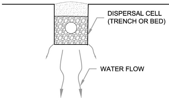
If the dispersal cell is located above a very low permeability layer, the water has to move to horizontally (sideways) to get out from underneath the dispersal area.
