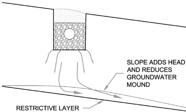
This groundwater mound continues to grow with time, and can reduce the VS below the system quite significantly. In many cases with poorly designed systems the mound will, over time, use up most of the VS.
