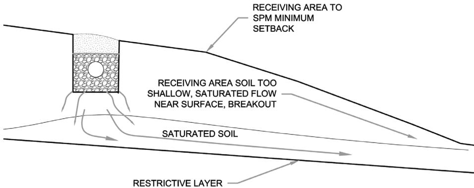
The capillary fringe is a problem here too—even if the water is near the surface contaminated water may wick up and cause a health hazard.
