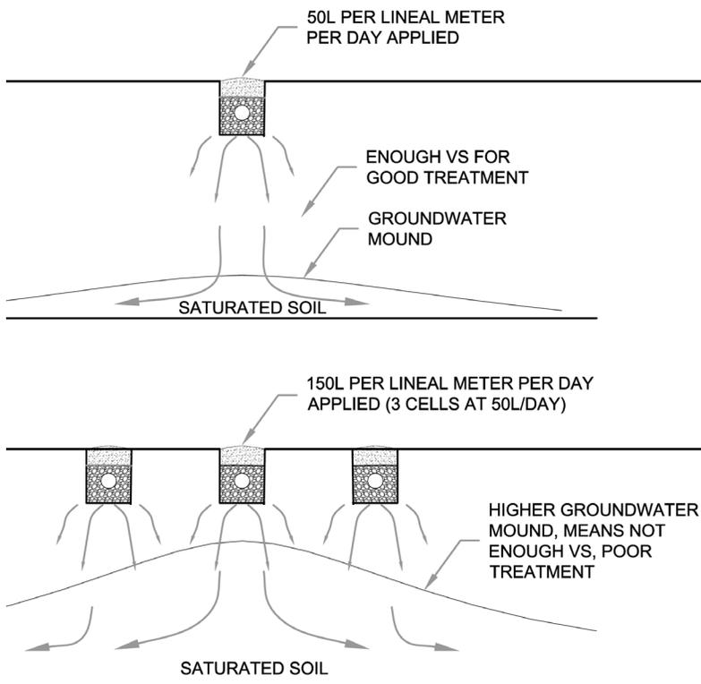
On a sloping site, the mound will be higher and also the amount of effluent flowing downhill per meter of contour length will be higher, and this may be too much for the available soil depth and head—resulting in breakout.
