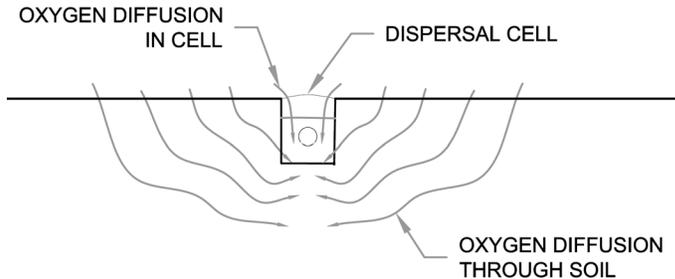
This oxygen has to diffuse through surrounding soil to get to the cell and to the soil below. This is not rapid; it is faster in dry soils and coarser soils. It is faster if the system is shallow so the oxygen has less distance to travel.
