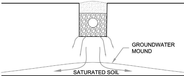
The head pressure drives the flow, and the finer the soil (with smaller pores) the more head is needed to drive the water through the soil, and so the higher the mound will become.
