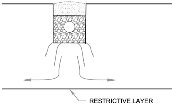
To move laterally, the water needs some head pressure to overcome the resistance to movement in the soil. On a flat site, this head can only come from the build up of a “mound” of groundwater under the dispersal area.
